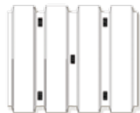
Type 1 slots / fissuration type 1
