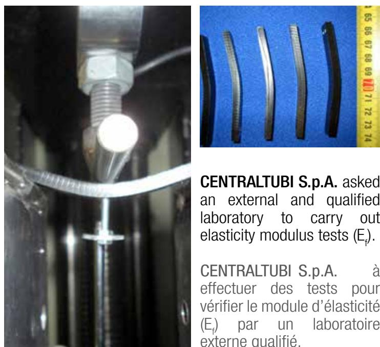
**CENTRALTUBI S.p.A.** asked an external and qualified laboratory to carry out elasticity modulus tests ( $E_f$ ).
