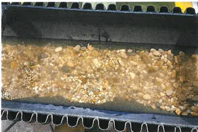
Figure 1: Sand/gravel/water mixture in the half shell before testing
