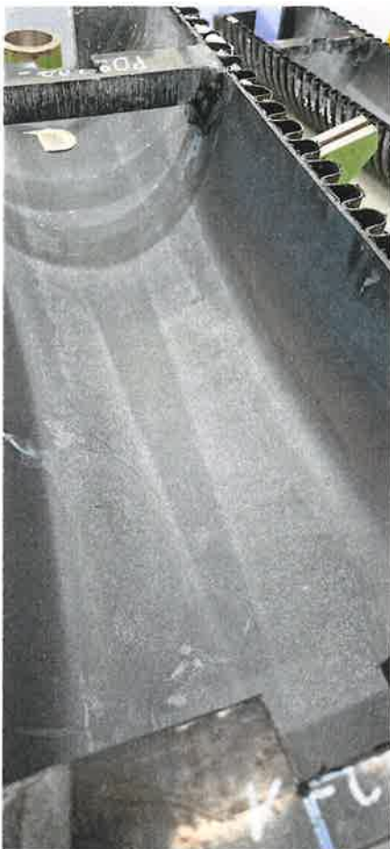
Figure 5: View into the half shell after 200,000 load cycles
