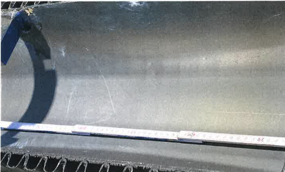
Figure 4: View into the half shell after 100,000 load cycles
