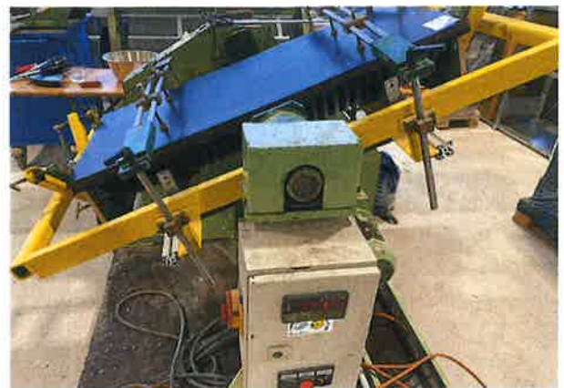
Figure 2: Testing in the Darmstadt tilting apparatus
